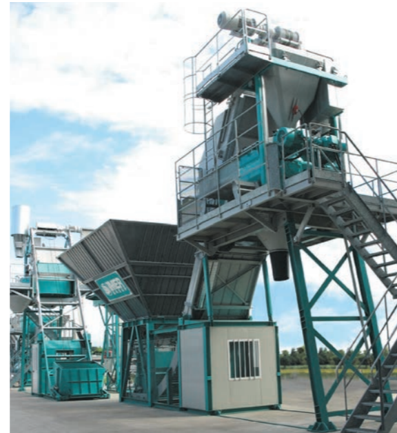
ORU ONEDAY MD concrete batching plant with aggregate storage, control cabin and incorporated weighing skip. Aggregates loading by payloader.
