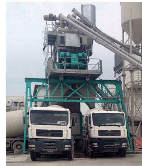
ORU DAY 150D mixing unit with built-in skip and cabin even during transport phases. Wider entrance to load several truck mixers thanks to the BYPASS system
