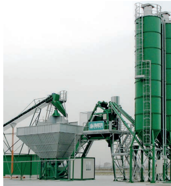
ORU ONEDAY MS concrete batching plant with aggregate storage, control cabin and incorporated weighing skip. Aggregates loading by conveyor belt.
